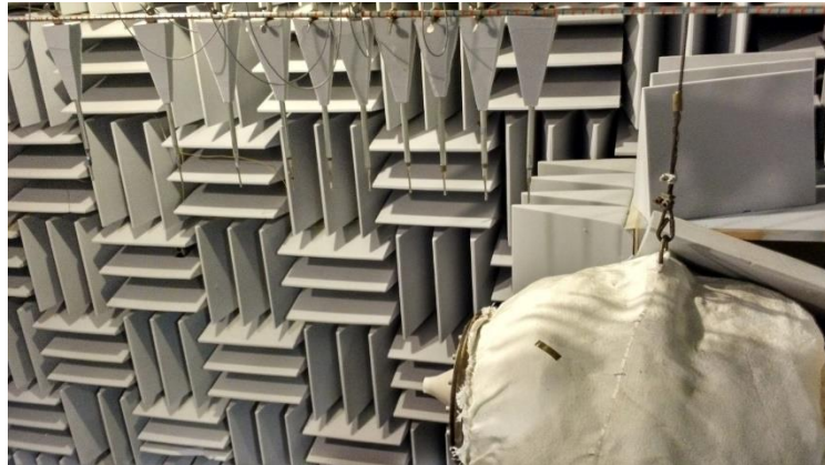
Figure 6.25: The near-field array in the GTRI Anechoic Jet-Facility.
